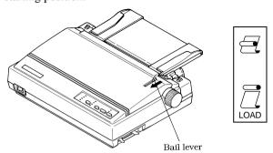
After the paper is fully fed (indicated by the printer's beeping), return the bail lever back to its original position toward the back of the printer.
